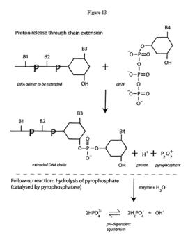
Genealysis, DNAe's underlying ISFET technology, operates by detecting changes in pH caused by the reaction of HIV genes on a specialized microchip.<sup>173</sup> The change in pH is sufficient to change the electrical state of the chip and turn it on. Thus, Genealysis uses these pH changes to identify the presence or absence of HIV in the blood by measuring pH changes related to HIV RNA and monitoring if the ART is working.
